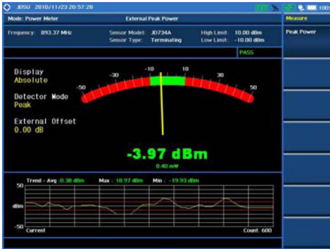
External Power Measurement
