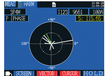
Harmonic power phase angle graph screen
