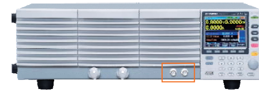
BNC connectors on the front panel
