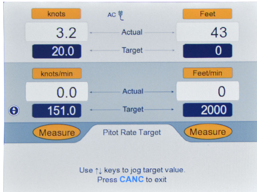
Figure 3.12 : Jog the Pitot Rate Target value
