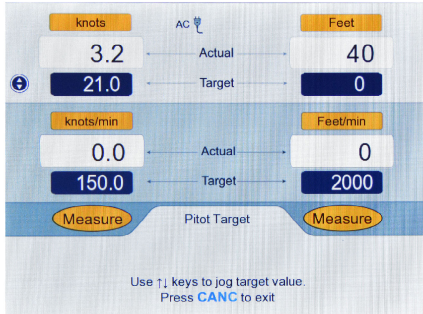
Figure 3.8 : Jog the Pitot Target value
