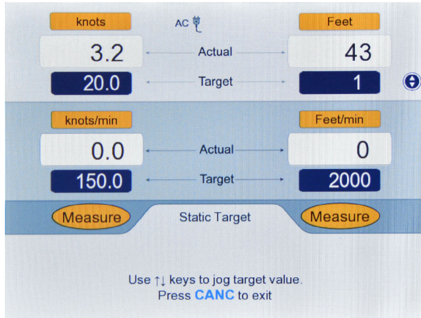
Figure 3.10 : Jog the Static Target value
