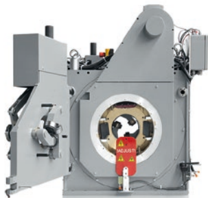
CIRCOSON® WT – EMAT technology for measuring wall thickness
